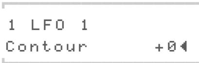
**Sine** Contour morphs from sine to a triangle wave (Contour to the left) or to a square wave (Contour to the right).
