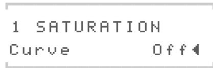
The display will read "SATURATION CURVE OFF", which means exactly what it says. With the VALUE buttons or the VALUE pot, you can now select from a number of *SATURATION*/distortion curves. Next to the distortion curves, the *SATURATION* stage offers further DSP effects such as the shaper, rectifier and filter. These are explained in detail in the section on the *SATURATION* stage.
