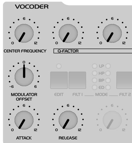
**Center Frequency** (Knob: *CUTOFF*, Default: 64 (middle)) The central frequency of the bandpass filters in the modulator- and carrier bank. Using a high Q (filter quality parameter, which is controlled using *KEYFOLLOW*) you can adjust the central frequency of the spectrum you edit.
