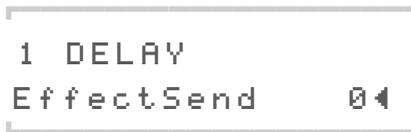
Here you will find parameters that are virtually identical to the parameters of the CHORUS group. Do not allow yourself to be confused by the slightly different terminology: The delay time is set via the parameter entitled *TIME* (equivalent to DELAY in the CHORUS section); the other features are FEEDBACK with a dedicated LFO and the familiar parameters RATE, DEPTH and SHAPE.
